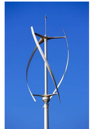
Figure 25: This photo is an example of a vertical axis wind turbine.
